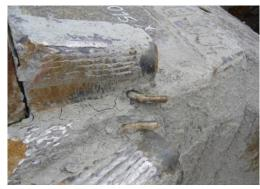
Fig. 4-5. Wrong positioning of the tooth adapters on the renewed buckets
