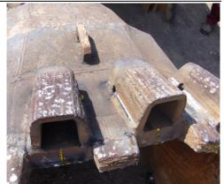
Fig. 6. Renewed cutting blade with adapters
